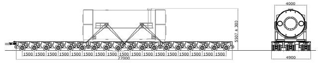
**Remarks:** (1) Overweight vehicle is composed of 18 axles of loading. (2) Total weight of trailer and cargo is 400 tons. (3) All Dimensions are shown in millimeters.
