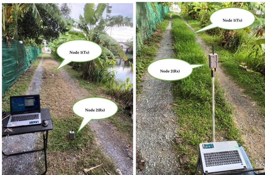
Figure 3. RSSI measurement for short grass (left) and tall grass (right).
