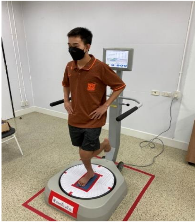
Figure 1. Motor Task. Single leg standing on unstable platform of Bio-Sway equipment to assess bio-sway indices represented a Motor Single Task.
