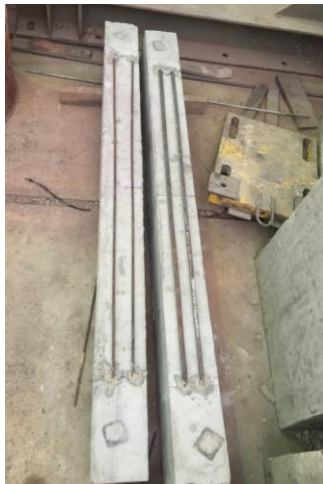
Figure 4. Installation of epoxy anchorage system
