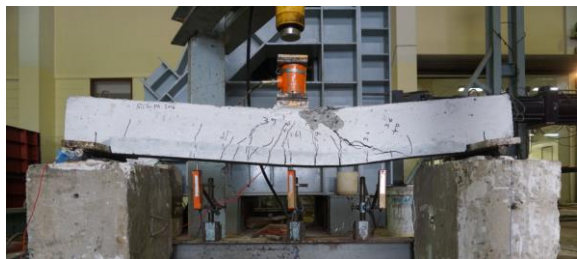
Figure 17. Failure mode of beam MEAS-6
