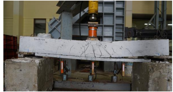
Figure 18. Failure mode of beam MEAS-10
