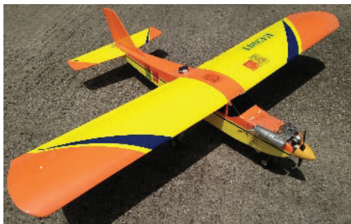
Fig. 5. Trainer aircraft c/w 0.55 cu in engine.
