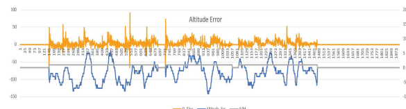
Fig. 10. Altitude's error and control output to elevator servo.
