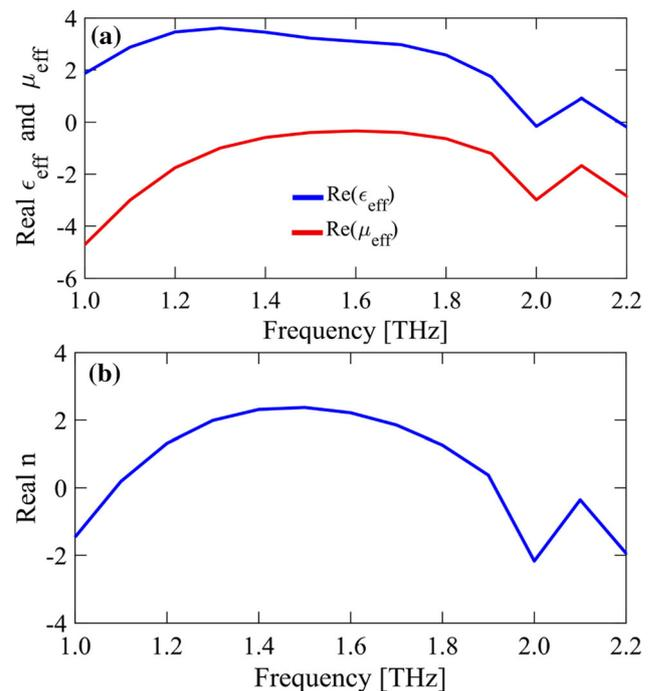
**Fig. 4** Results of the Matlab program, where **a** real permittivity and permeability, **b** real refractive index where the resonance frequency is 2THz
