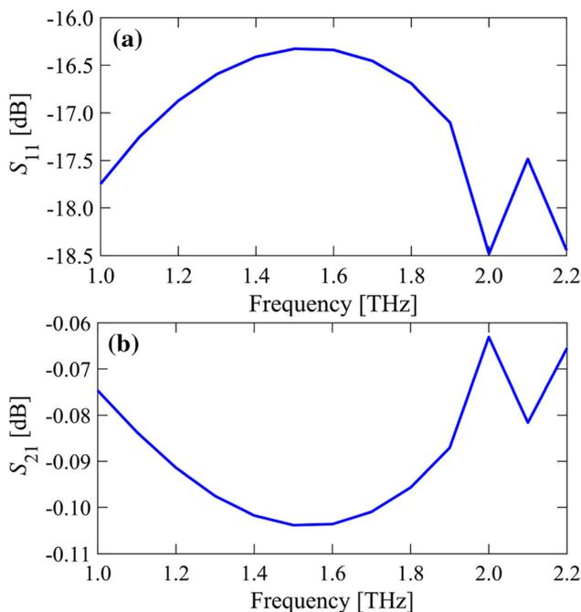
**Fig. 3** Plots of the S-parameters extracted from the HFSS software, where (a) reflection coefficient, (b) transmission coefficient where the resonance frequency is 2THz and 2.10THz, respectively
