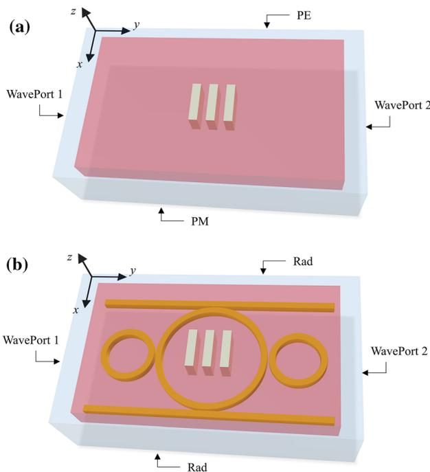
**Fig. 2** Illustration of the HFSS structure, where **a** Silver bars at the center of the silicon substrate inside the radiation box with perfect electric (PE) and magnetic (PM) boundary conditions, **b** Silver bars at the center ring inside the radiation box with radiation (Rad) boundary condition
