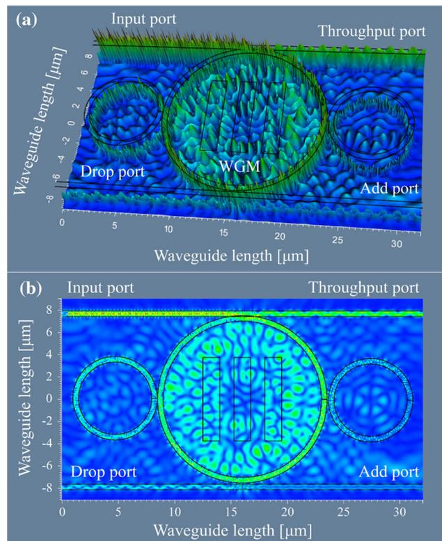
**Fig. 8** Shows the Optiwave results of the system in Fig. 1 using the selected parameters in Table 1, where **a** whispering gallery mode formed at the center ring, where WGM, **b** electric field distribution across the system
