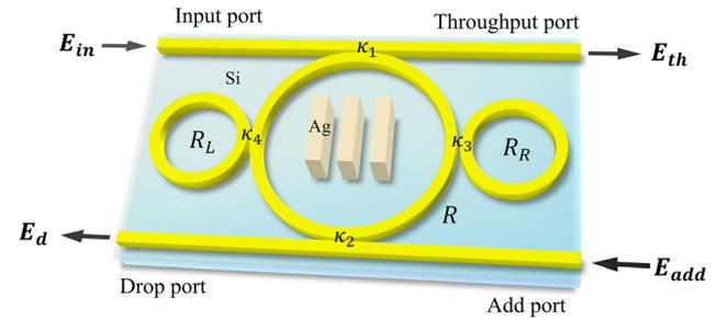
**Fig. 1** Illustrates the fabrication structure of the micro-metamaterial antenna, where  $E_{th}$  is defined as the throughput port,  $E_d$  is defined as the drop port,  $E_{add}$  is defined as the add port,  $E_{in}$  is defined as the input port.  $\kappa_1$ – $\kappa_4$  are the coupling coefficients
