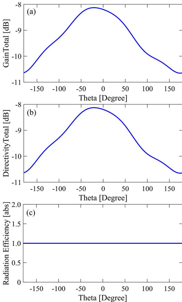
**Fig. 7** The plot of **a** the total gain of the antenna, **b** the total directivity of the antenna, and **c** the radiation efficiency of the antenna. The gain and directivity is -8.13 dB while the radiation efficiency is 1
