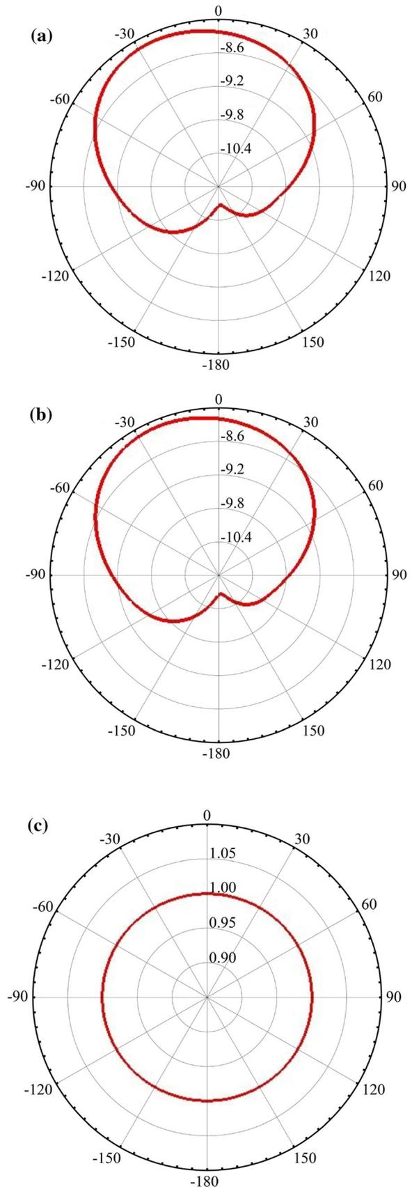
**Fig. 5** Plots of the antenna S-parameters extracted and plotted using the Matlab program, where (a) the reflection coefficient, (b) transmission coefficient. Both having a resonance frequency of 1.60THz
