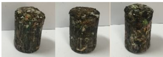
Figure 2: The RDF with PVA as binder at 20 %wt.
