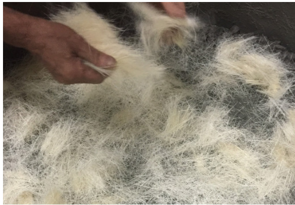
Fig. 2 Mixing procedure of sisal fiber reinforced concrete.
