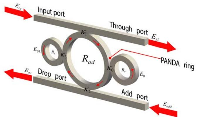
FIG.1 THE MODIFIED ADD/DROP RING RESONATOR
