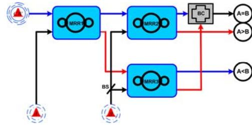
**FIG. 6** ALL-OPTICAL DATA COMPARISON
