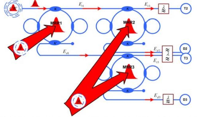
FIG.3 RING RESONATOR CIRCUITS FOR ALL-OPTICAL LOGIC AND ARITHMETIC OPERATIONS OPTICAL BASE TREE ARCHITECTURE
