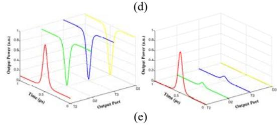
**FIG.5** SIMULATION RESULTS OF THE OUTPUT LOGIC GATES WHEN THE INPUT LOGIC STATES ARE (B) 00 ‘DD’, (C) 01 ‘DB’, (D) 10 ‘BD’ AND (E) 11 ‘BB’.
