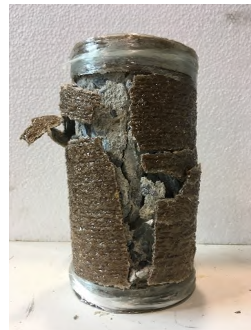
Fig. 7. Typical failure mode of RE-1 specimen.
