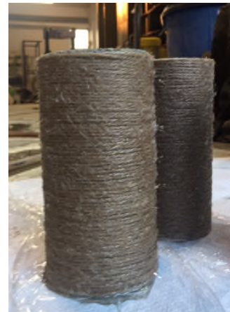
Fig. 4. Typical RFRP strengthened specimen.
