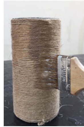
Fig. 3. Applying the epoxy resin using resin
