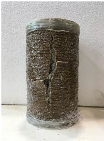
Fig. 8. Typical failure mode of RE-2 specimen.
