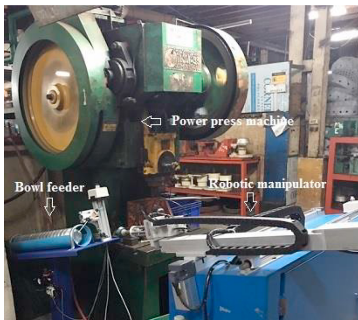
Fig. 10. The loading/unloading system
