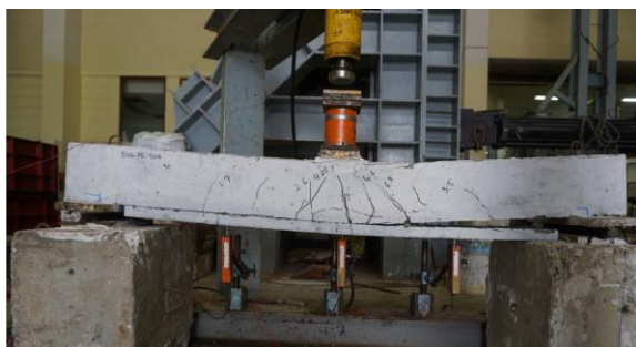
Figure 18. Failure mode of beam MEAS-10
