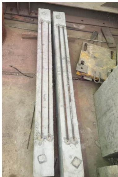
Figure 4. Installation of epoxy anchorage system
