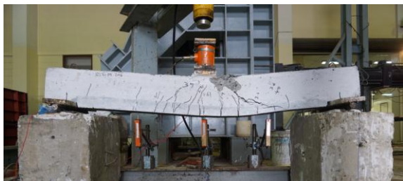
Figure 17. Failure mode of beam MEAS-6
