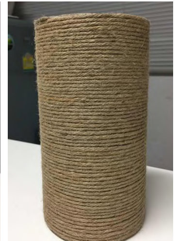
Fig. 3. A typical rope strengthened concrete specimen.
