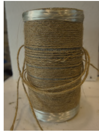
Fig. 5. Typical failure mode of R-1 specimen.
