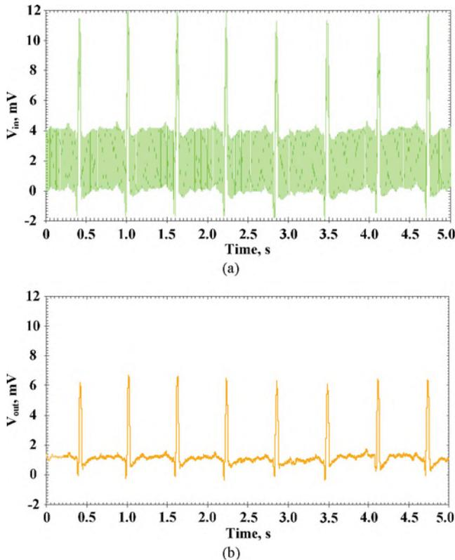
Fig. 12. Transient response of fifth-order Butterworth low-pass filter for ECG signal: (a) input, (b) output.
