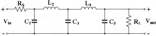
Fig. 8. Fifth-order low-pass RLC ladder filter.
