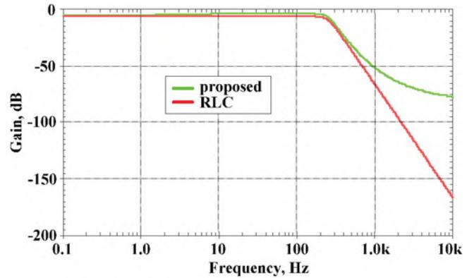
Fig. 9. The magnitude response of fifth-order Butterworth low-pass filter.
