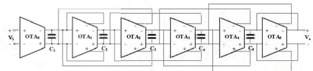
Fig. 2. Fifth-order Butterworth low-pass filter using MODI OTAs [7].
