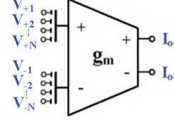
Fig. 5. Symbol of multiple-input OTA.
