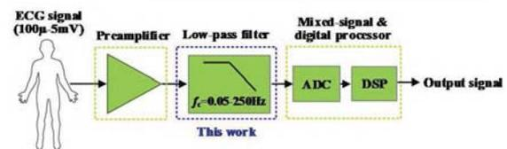
Fig. 1. ECG acquisition system.
