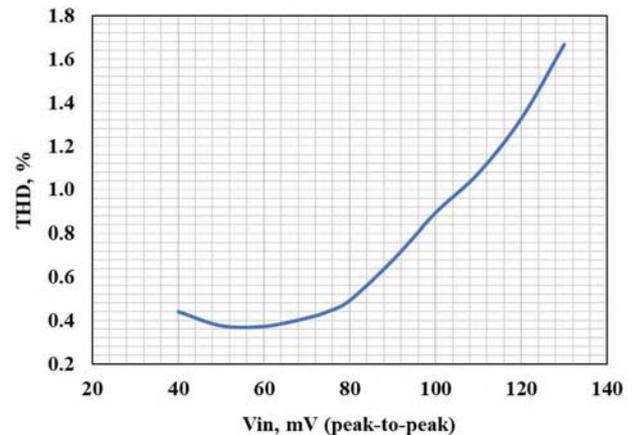
Fig. 11. The harmonic distortion of propose circuit.
