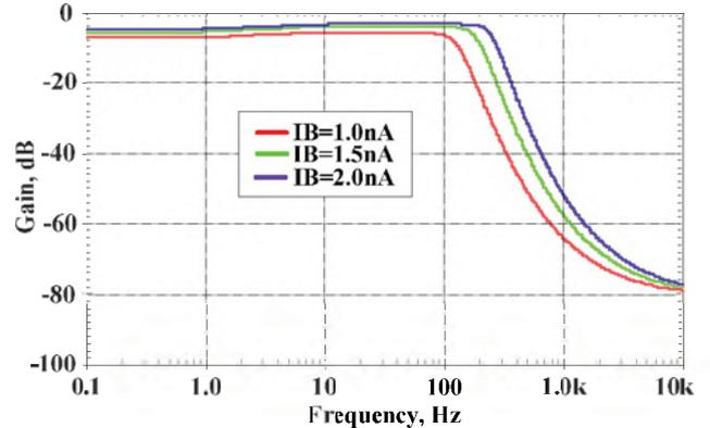
Fig. 10. The magnitude response of filter with different bias currents.
