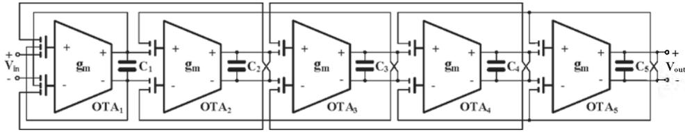
Fig. 7. Proposed fifth-order Butterworth low-pass filter using MI-OTAs.
