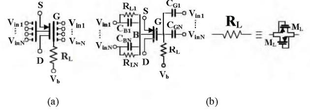
Fig. 4. MIBD-QFG MOS transistor, (a) symbol, (b) realization.
