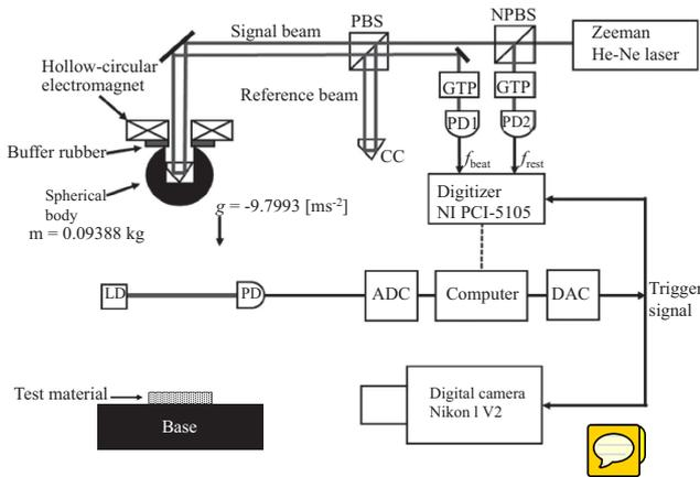
**Fig. 1.** A schematic diagram of the experimental setup (NPBS=Non-polarized beam splitter, PBS=Polarized beam splitter, CC=Cube corner prism, GTP=Glan-Thompson prism, PD=Photo detector, LD=Laser diode, ADC=Analog-to-digital converter, DAC=Digital-to-analog converter).
