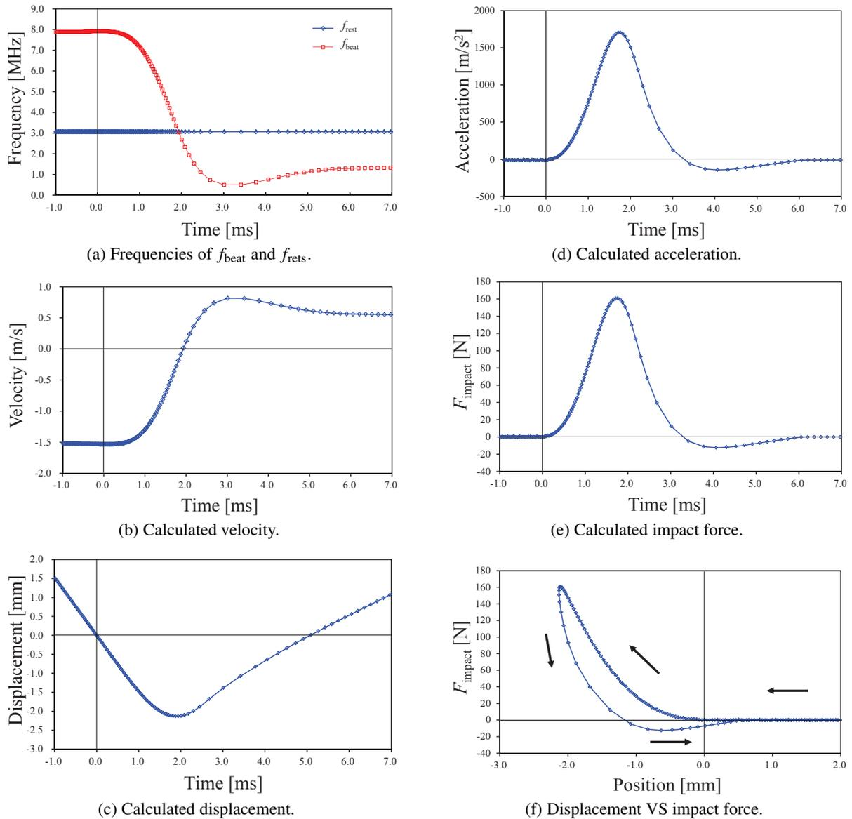
**Fig. 2.** (a)–(f) Data processing procedure: calculation of velocity, position, acceleration, and force from frequency which the details are as follows: maximum impact force:  $1.60 \times 10^2$  N, contact time: 6.2 ms, velocity before impact:  $-1.53$  m/s, velocity after impact:  $0.56$  m/s, coefficient of restitution: 0.36, and energy loss:  $9.5 \times 10^2$  J (87%).
