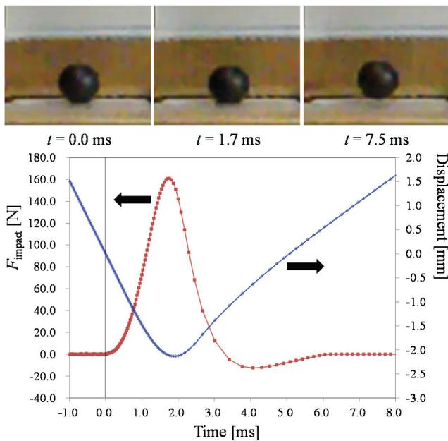
Fig. 4. Changes in impact force and displacement against time.
