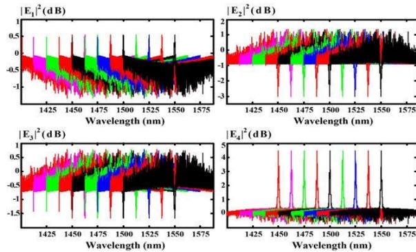
Fig. 3. Many soliton spins within a PANDA ring are generated using a dark-soliton pump input at center wavelength 1400, 1425, 1450, 1475, 1500, 1525, 1550, 1575, and 1600 nm.
