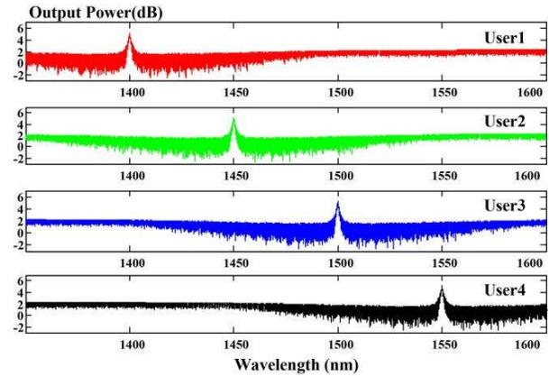
Fig. 7. Shows the results that received by each user 1-4 from add-drop filter at Drop port.
