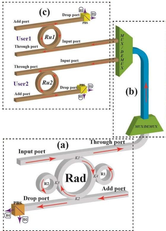
Fig.5. A schematic diagram of spin distributed networks using the multi-wavelength optical spins, where Di: detectors, PBS: polarizing beam splitter, Rgs: output ring radii (users)
