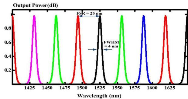
Fig. 8. Simulated transmission FSR= 25 nm and FWHM = 4 nm.
