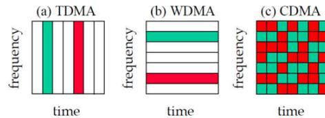
Fig. 1. Time-frequency space usage in (a) TDMA, (b) WDMA, (c) CDMA
