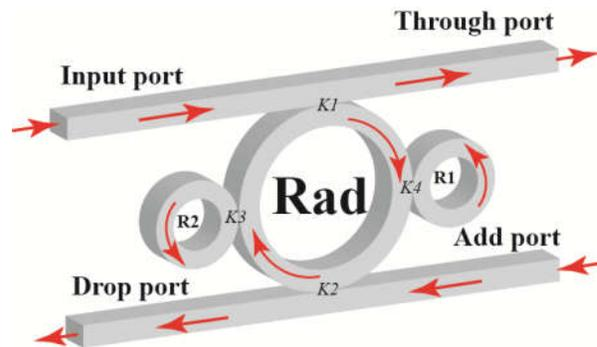
Fig. 2. The Panda Ring Resonator
