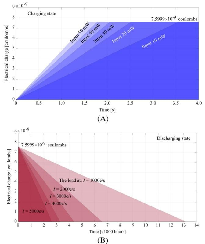
**FIGURE 4** Results of the induced electrical charge characteristics using the proposed circuit, A, the charging state, where the input light powers are varied from 10 to 50 mW, and B, the discharging state, where the loads are varied from 1000 to 5000 e/s [Color figure can be viewed at [wileyonlinelibrary.com](http://wileyonlinelibrary.com)]
