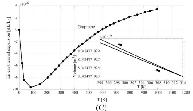
**FIGURE 3** Thermal expansion of the island rings-silicon, graphene, gold, where A, and B,<sup>11</sup> C<sup>12,13</sup> [Color figure can be viewed at wileyonlinelibrary.com]
