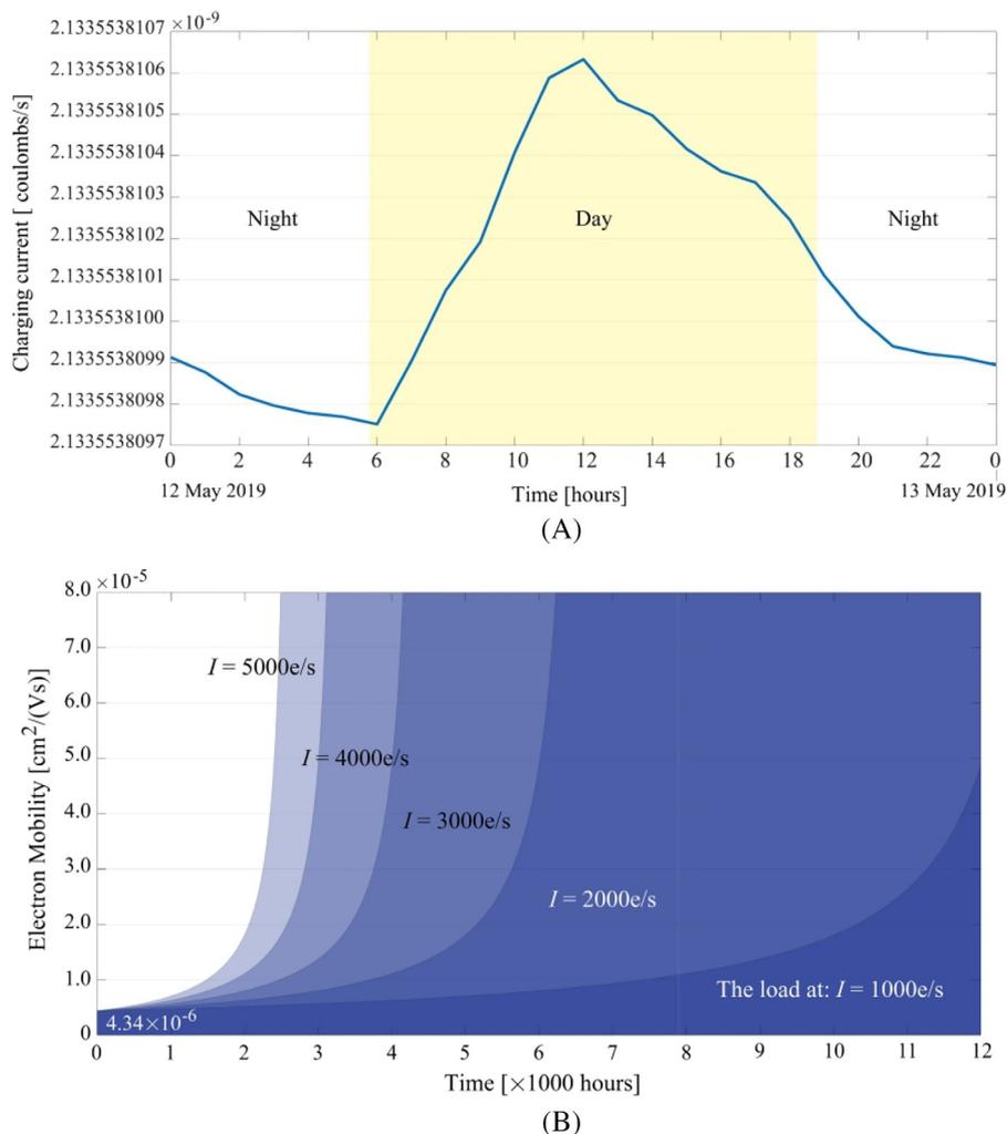
**FIGURE 5** In manipulation, the thermal expansion is employed by the relationship between the input light power and the induced electron mobility, where A, the reference to a weather data record,<sup>17</sup> B, the daily charging current for the input light power of 10 mW can be obtained as in the figure, from which the electron mobility of  $4.34 \times 10^{-6} \text{ cm}^2/(\text{V}\cdot\text{s})$  can be obtained [Color figure can be viewed at wileyonlinelibrary.com]
